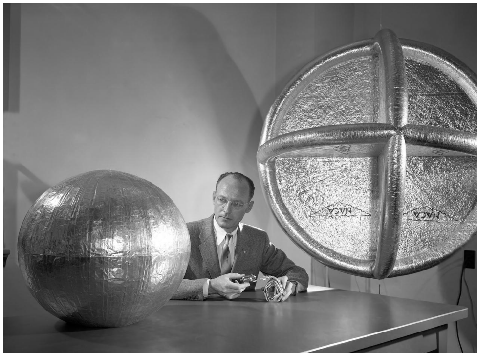
Figure #13. Engineer W.J. O'Sullivan, Jr. with a 20 Inch Sub satellite (Courtesy of the National Aeronautics and Space Administration).
