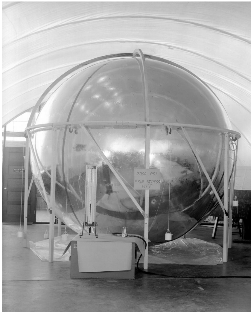
Figure #11. A scale prototype of an Echo Satellite, 12 feet in diameter (Courtesy of the National Aeronautics and Space Administration).
