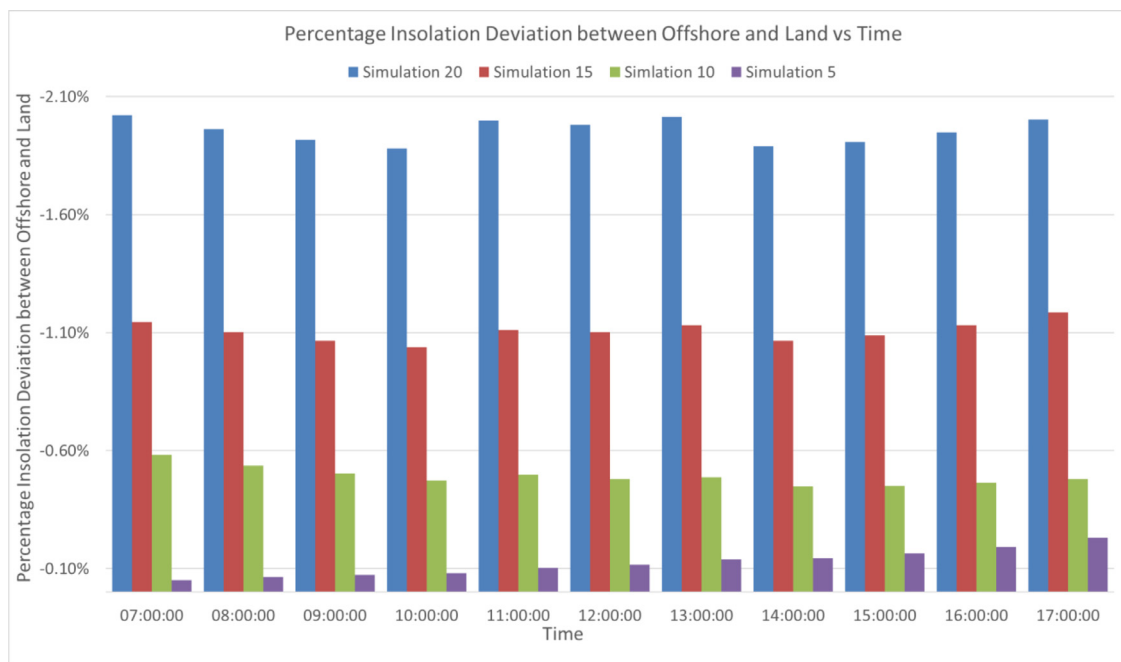
Fig. 14. Percentage insolation deviation of offshore from land due to roll movements (13/06/2019, \beta = 5^\circ , Fixed \alpha = 0^\circ ).
