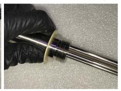
3-Piece Filter Cap Assembly required - installation of O-ring - probe fully inserted into heater assembly:
