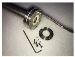
Probe Flange Gasket removal - flange gasket installation onto probe - slid to the front surface of flange:
