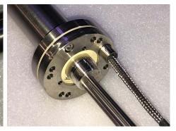
Retaining Ring installed - secured by 3 cap screws - side view showing the normal gap of retaining ring:
