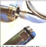
3. In-situ diluting probe tip, with special grooved filter cap for the Kalrez o-ring.
