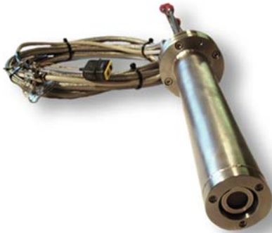
1. Coil assembly with inner flange flange removed from mantle.
