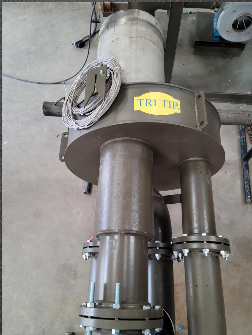
D.B.I.'s "Tri Tip®" will accept three independent pressure streams in one tip with one ignition system.
