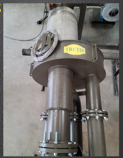
D.B.I.'s "Tri Tip®" will accept three independent pressure streams in one tip with one ignition system.
