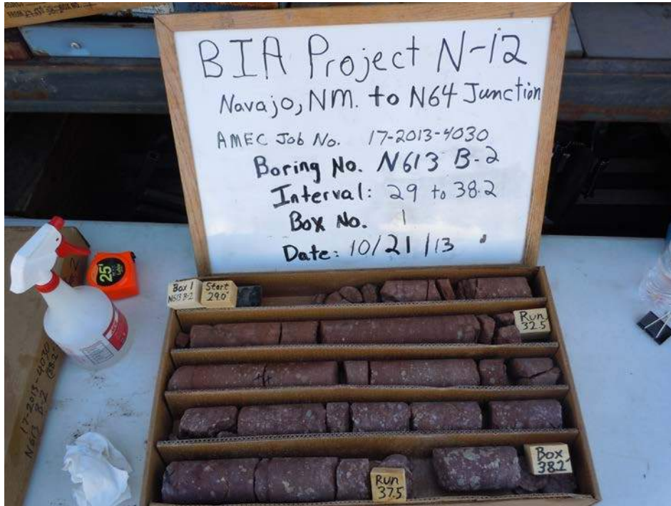
Photograph No. 25 Bridge N613, Boring No. 2, 8.84 meters to 11.64 meters
