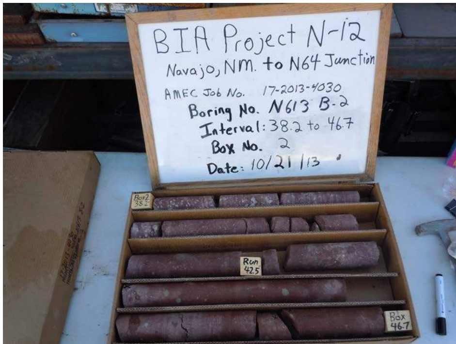
Photograph No. 27 Bridge N613, Boring No. 2, 11.64 meters to 14.23 meters
