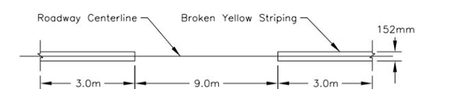
TYPICAL PAVEMENT MARKING "BROKEN YELLOW"
