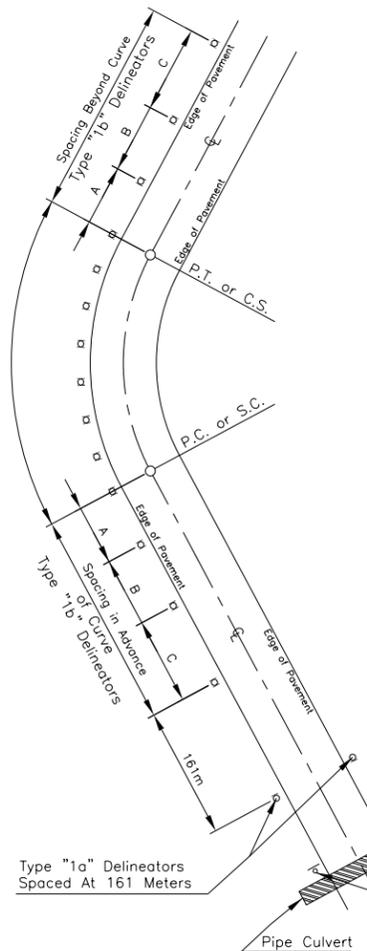
Type "1a" Delineators Spaced At 161 Meters
