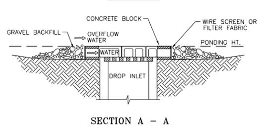
**BLOCK AND GRAVEL DROP INLET SEDIMENT BARRIER**
