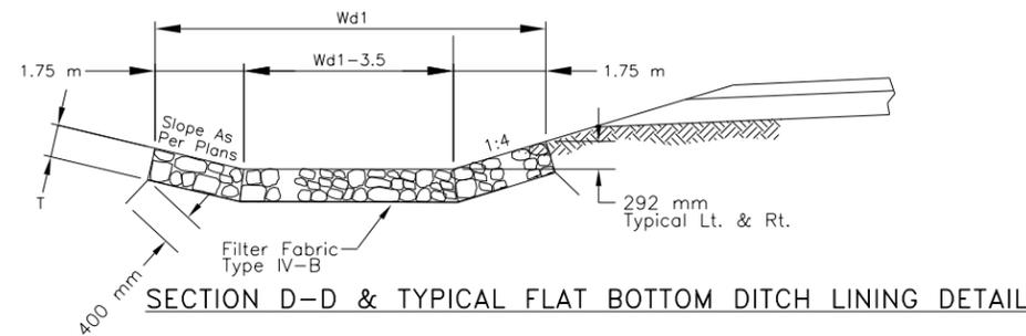
SECTION D-D & TYPICAL FLAT BOTTOM DITCH LINING DETAIL
