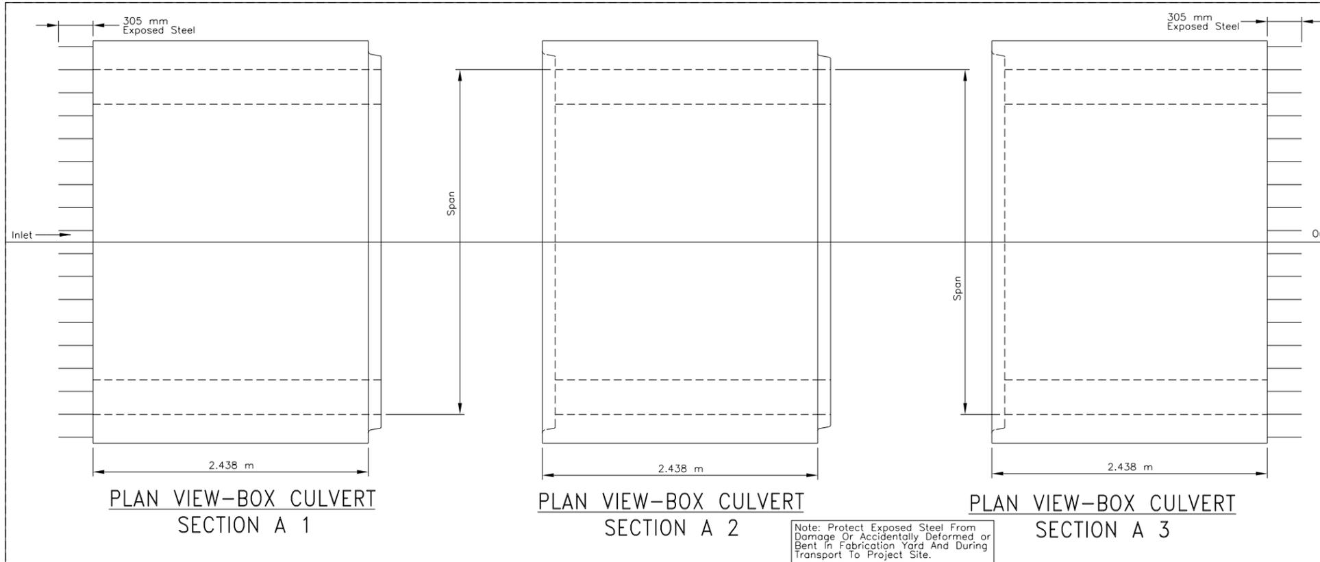
**STANDARD PRECAST BOX CULVERT DESIGNS (51 mm COVER) - 2.438 m, 3.048 m & 3.658 m SPANS**
