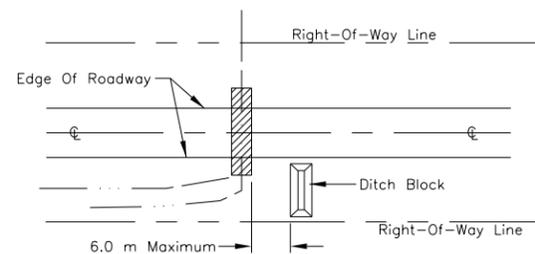
**DITCH BLOCK INSTALLATION AT STRUCTURE**
