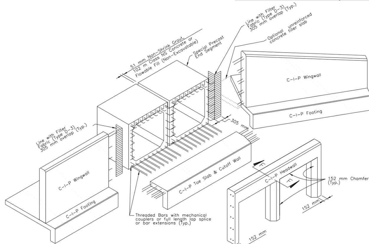
**EXPLODED VIEW OF CONNECTIONS AT END OF CULVERT**
