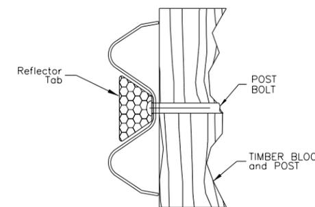
**SECTION REFLECTOR TAB MOUNTING DETAIL**
