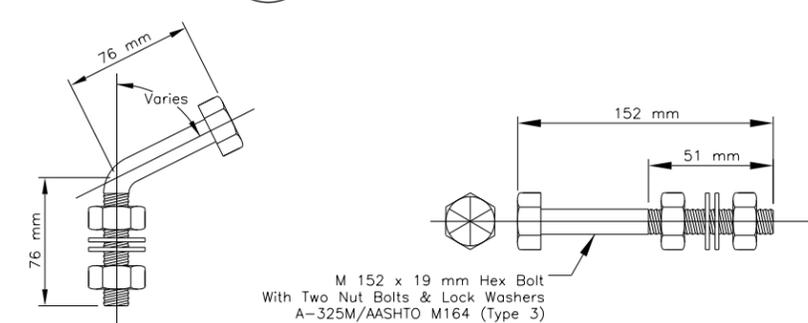
\*NOTE: Anchor Bolts Shall Be Bent/Fabricated As Needed to Align With The Concrete Slope Blanket Prior To Bolting To The Culvert. The Culvert Wall Shall Not Be Deformed/Bent To Align Bolts
