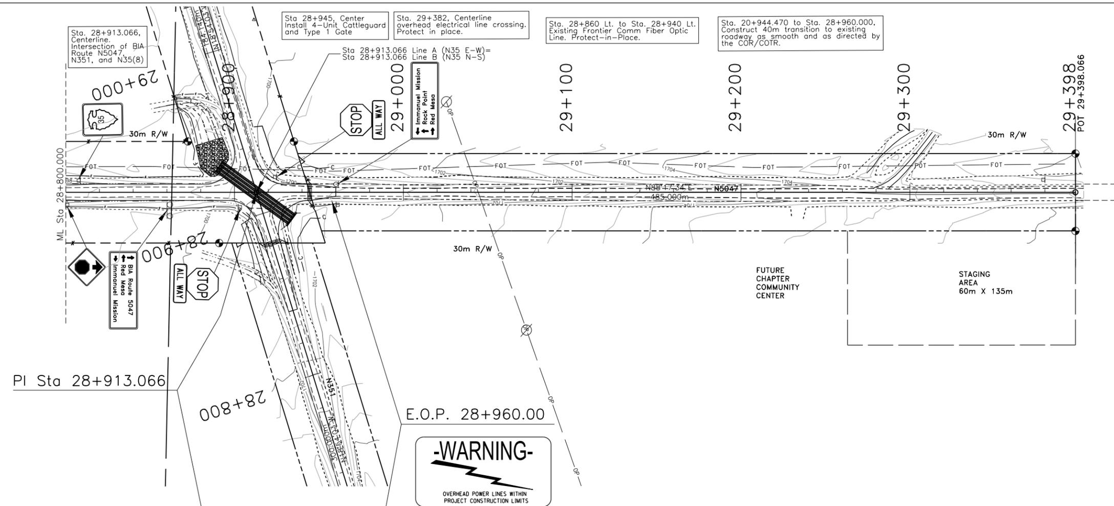
Grade & drain transition ditch from new ditch flow line (Sta. 28+948.470) Left & Right to existing road ditch flow line in 100m or as directed by the COR/COTR. This work shall be incidental to the earthwork bid items.
