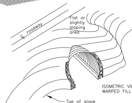
**PIPE SKEWS TO THE EMBANKMENT WARPING (TYP.)**
