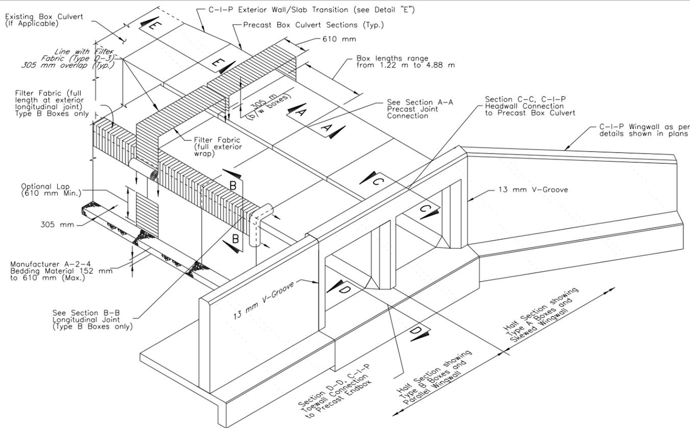
**ISOMETRIC VIEW OF PRECAST CONCRETE BOX CULVERT**
