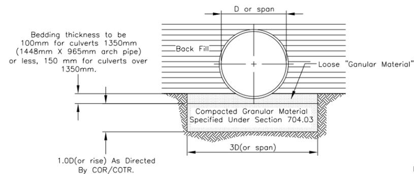
**FIGURE C: FOUNDATION STABILIZATION BEDDING**
