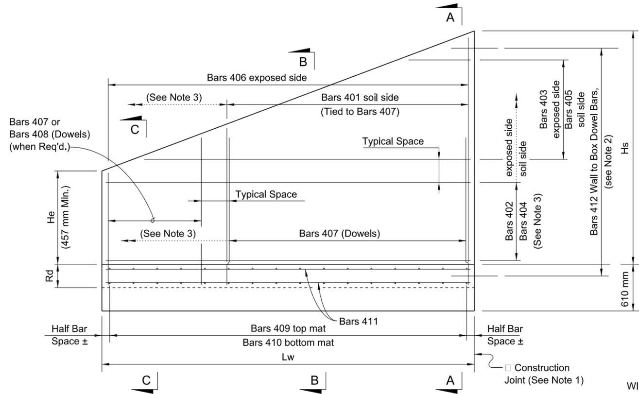
WINGWALL ELEVATION - Variable Height
