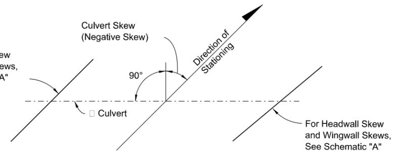
SCHEMATIC "B" - PLAN VIEW CULVERT ALIGNMENT
