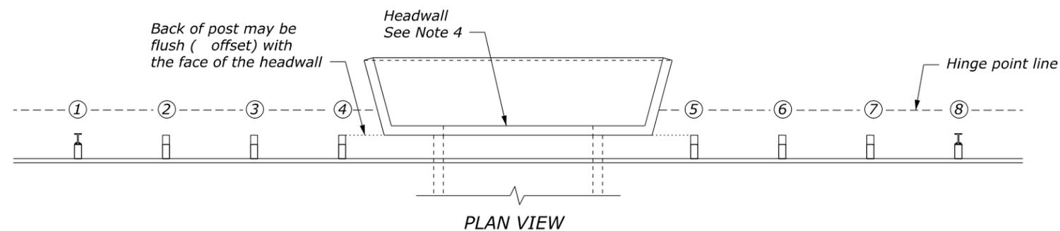
**SPAN WITH HEADWALL DETAIL**
