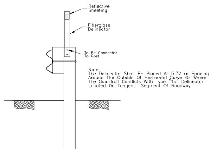
**ELEVATION GUARDRAIL/POST MOUNTED DELINEATOR (TYP.)**
