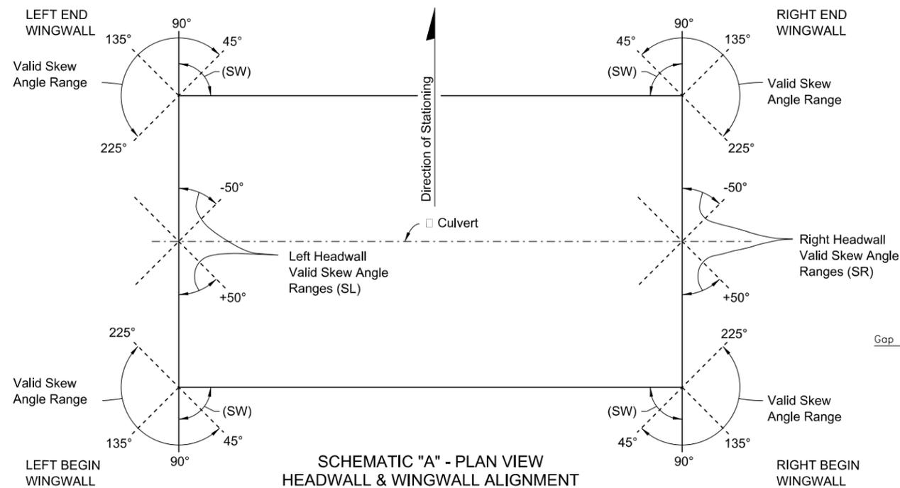
NOTE: All headwall and culvert skew angles are measured in degrees from a line perpendicular to the centerline of culvert (counter-clockwise positive), see Schematic "B".
