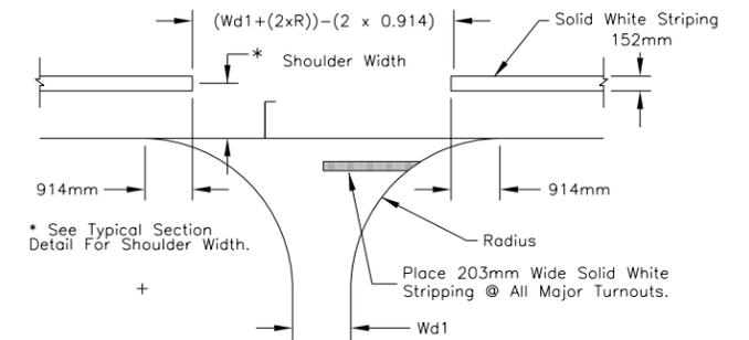
TYPICAL PAVEMENT MARKING @ TURNOUT
