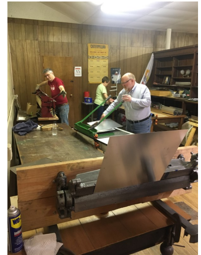
Volunteers at the Raymond workshop bend sheets of metal into bread pans to be included with each oven.
