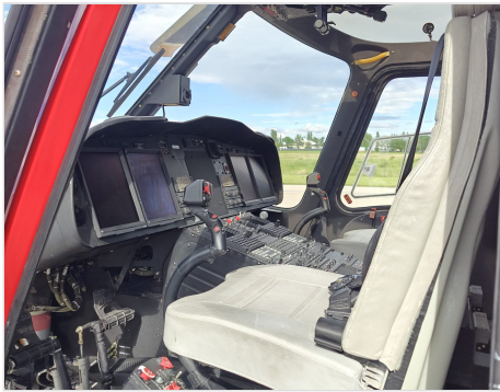
Cockpit — Honeywell Primus EPIC integrated flight deck • 12-passenger utility cabin
