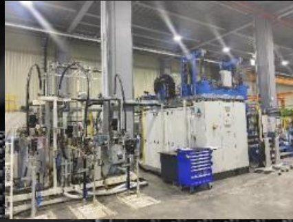
HP-RTM (The only ultra-high-pressure injection machine in Taiwan)
