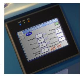
A touch screen allows users to select preset protocols or design new ones. The screen can be controlled remotely using an Internet connection.
