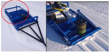
Note: make sure the weights are no larger than 10" in diameter as they will contact the rear cross member damaging the track setter
