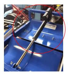
> ALWAYS DISCONNECT THE ELECTRIAL CONDUCTOR TO THE ELECTRICALLY ACTUATED TRACK SETTER WHEN UNHOOKING FROM THE TOWING MACHINE.
