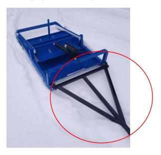
Install the Tow Bar with supplied lynch pins. Ensure washers are installed. Use a soft face hammer to drive the pins out and in as they are a snug fit.
