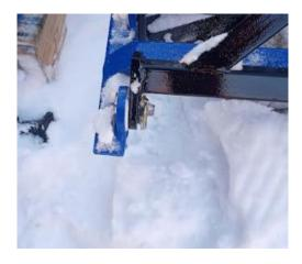
• Set the Tow Bar in position and reinstall the Tow Bar Pins. Again, use a soft face hammer to drive the pins back in place through the Tow Bar clips. Put the washer over the pin and reinstall the 3/16" lynch pins.
