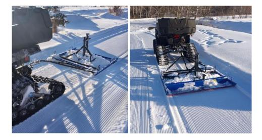
• Do not be alarmed with snow build up on top of the Renovating Leveler. In fact, it adds more weight and produces better results.
