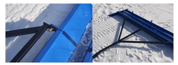
• Set the Tow Bar in position and reinstall the Tow Bar Pins. Again, use a soft face hammer to drive the pins back in place through the Tow Bar clips. Put the washer over the pin and reinstall the 3/16" lynch pins.
