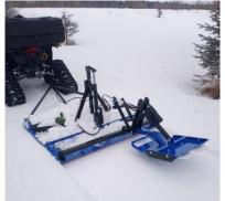
• If the TnT is equipped with a wheel kit, it is recommended to leave the Tow Bar Retaining Bar engaged, making the Tow Bar a rigid member and keeping the Renovating Leveler in a more level plane while grooming.
