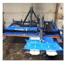
• Connect the electrical conductor quick connect of the Actuator to the cable from the Junction Box.
