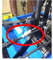
• Install the Tow Bar with supplied lynch pins. Ensure washers are installed.
