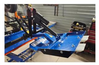
• Connect the electrical conductor quick connect of the Actuator to the cable from the Junction Box.
