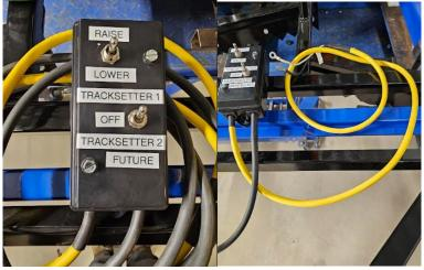
ATS has labelled the actuator control pendant accordingly for simplicity.
