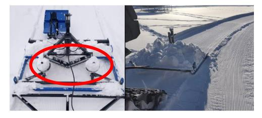
Maximum recommended towing speed for packing and leveling is 5 to 10 kpm. For best results, the slower the better.
