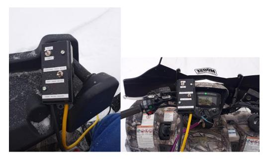
The Yellow conductor cable goes to the power source. The black wire gets connected to the
