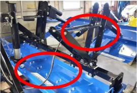
• Install the Tow Bar with supplied lynch pins. Ensure washers are installed.
