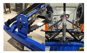
For optimal leveling and renovating results when working hard packed or icy snow, the Renovating Leveler should have 100-200 lbs of weight added on the weight pins. Allowing snow to accumulate on top of pan adds weight as well.
