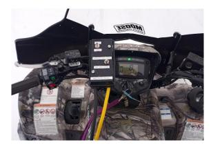
• Feed the TnT black power conductor cable to the back of the tow machine.
