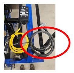
• Secure socket on the black power conductor to the back of the tow machine.
