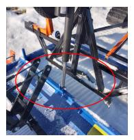
6. Remove the Wheel Arm Lock Pins from the Lock Pin Holes on each Wheel Support Arm (may need to tap when a soft hammer).
