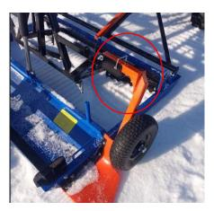
9. Lower the Cutting Bed with the Electric Actuator to raise the Renovating Leveler off the ground for traveling. You do not lower Cutting Bed any lower than necessary, but just high enough to give you adequate ground clearance.
