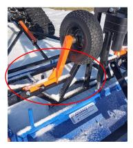
7. Lower the Wheels by rotating the Wheels and Support Arm until wheels are facing ground. Downward. You may have to raise the Cutting Bed higher if wheels will not swing completely down.
