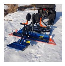
14. Lower the Cutting Bed to the ground using the Jack for grooming.
