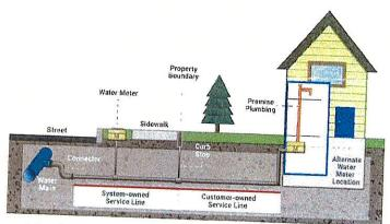
A service line is defined as the pipe that connects the water main to a building's inlet. Classification of the entire length of each service line is required, regardless of ownership or use.
