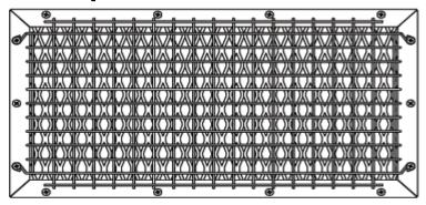
The catalyst assembly including—front bezel plate, expanded metal, protective scrim cloth, and catalyst mat can be quickly disassembled by removing the fourteen (14) 1/4" x 20 Hex head bolts and replacing with a brand new one. The spent core can be returned to Advanced Catalyst Systems, LLC for a core charge credit. No more downtime due to shipping failed heaters to the factory. Available in standard and custom sizes.
