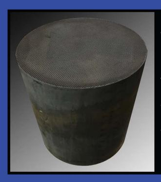
ACS' Catalyzed DPF's oxidize CO, VOC, and HAP's while filtering out harmful particulate matter (PM). ACS' DPF's are used extensively in mobile and stationary applications across the world. Proprietary catalyst formulations provide low regneration temperature and excellent destruction rate efficiencies for criteria pollutants. Available in standard sizes and cell geometries.
