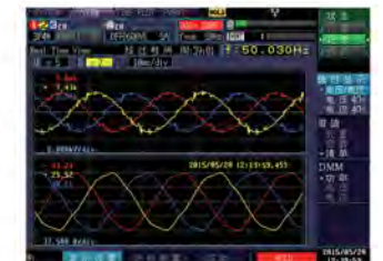
Voltage and current in the metallurgical industry after governance
