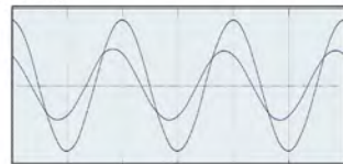
SVG emits capacitive reactive power, which is offset by inductive reactive power, and the voltage and current are in phase.
