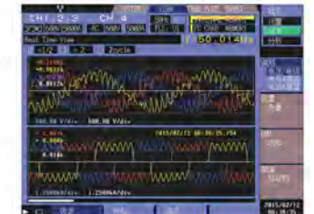
Voltage and current in the metallurgical industry before governance
