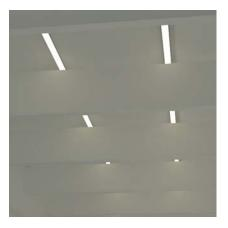
Hanging acoustic baffling throughout the train significantly reduces the amount of ambient noise on the train and diffuses direct lighting from the LED strips above by narrowing the amount of light that is visible at further distances.
