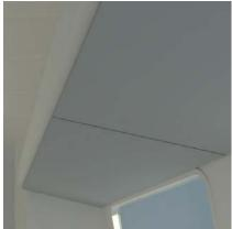
Sound panels beneath the overhead storage optimizes the ability for small groups of people to have quiet conversations, filtering out exterior noise and limiting reverberation throughout the café, the most heavily occupied space on the train.
