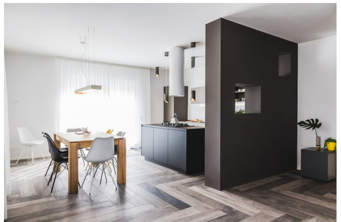
DOMESTIC TACTILE FLOORING | Designed for a blind client, the flooring uses stone and porcelain to embed a glyphic map of the circulation in the house. (So & So Studio, 2018).
