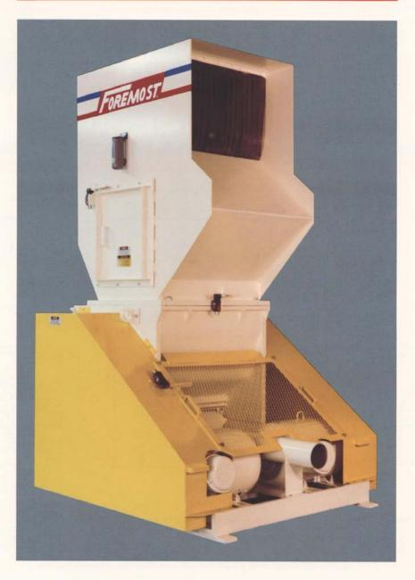
The HD-8 scrap grinder is specifically designed and built to granulate either large parts or high volumes of scrap material. With its large throat size of 24" x 36", offset cutting chamber and rugged construction, large molded parts can be readily granulated without the need for pre-cutting. It is an ideal machine for applications such as post consumer scrap recycling when equipped with our optional high throughput rotor and screen package.
