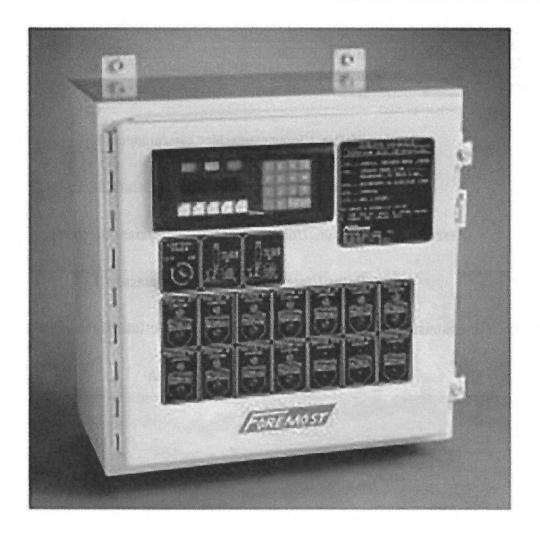
The Format IV is a user-friendly PLC based vacuum loading system controller. The Format IV has the capability of controlling up to 3 vacuum pumps and 27 loading stations in any combination of pumps and stations as required.
