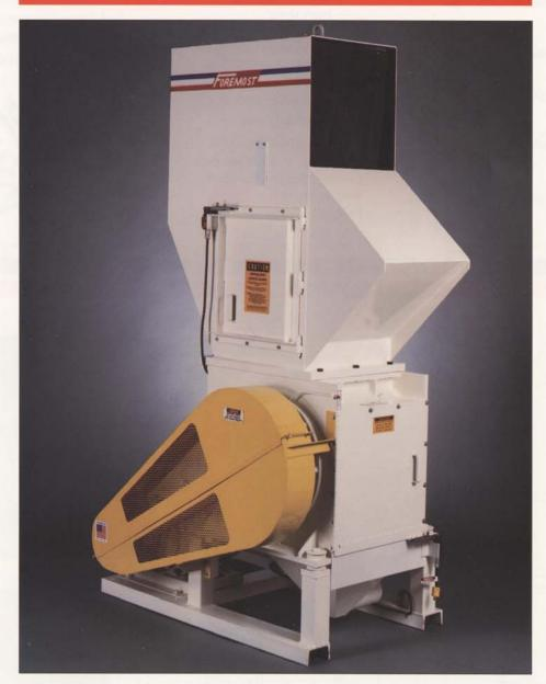
The LD-7 scrap grinder is specifically designed and built to granulate either large parts or high volumes of scrap material. With its large throat size of 24" x 24", offset cutting chamber and rugged construction, large molded parts can be readily granulated without the need for pre-cutting. This grinder features a standard two-bladed rotor.
