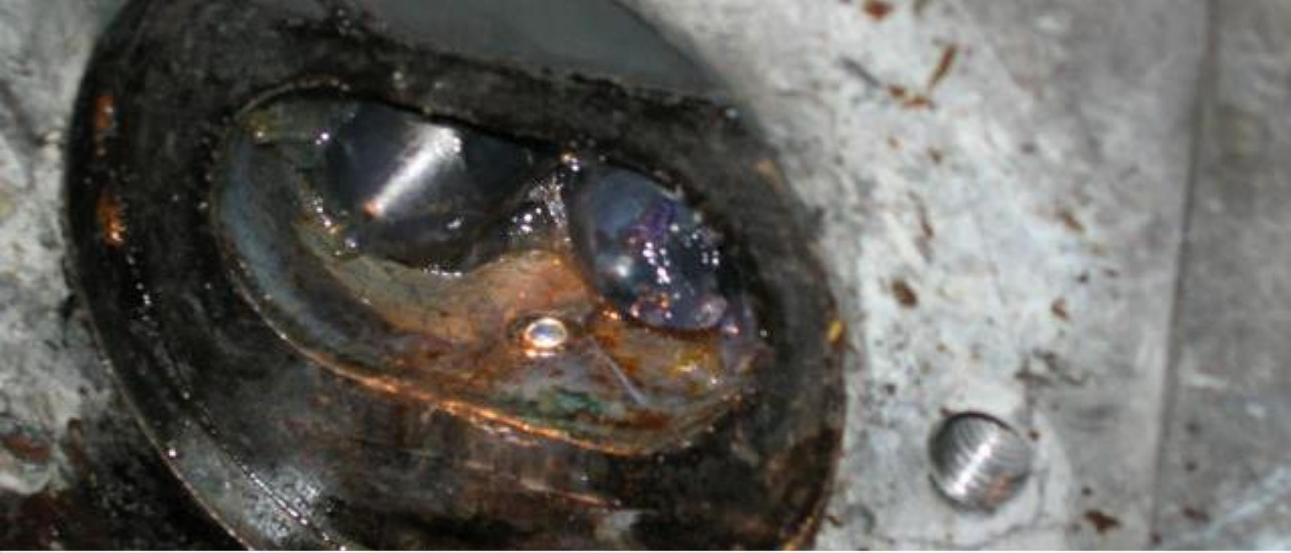
Reflection Polymer Melt Probe
