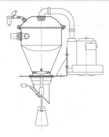
Foremost centrifugal blowers offer inexpensive, low, maintenance alternative to positive displacement pump type vacuum loading system. Available in 1.3 and 2.0 HP Models.
