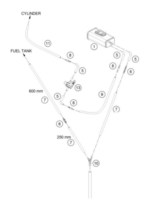
STEP 1: Remove the fuel tank according the owner's manual. Locate the EVAP Valve (13), the pipes and the EVAP system canister (1) as shown in the diagram.
