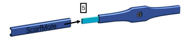
Step 5: With the ScarfMate logo facing forward, slide front bar connector over back bar connector until 2<sup>nd</sup> circle snaps into place
