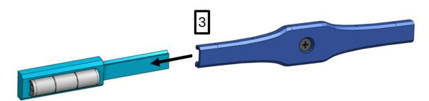
• Step 3: Remove Level Holder from middle piece to prepare for insertion of next section
