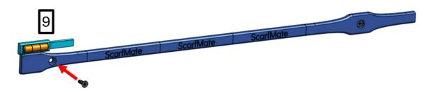
• Step 9: Insert provided anchor into hole on end piece & fasten it to the wall until anchor bottoms out in the back of the middle connector. You can also place the level on top of end piece to ensure it is level.
