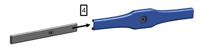
• Step 4: With the (2) circles facing forward, insert back bar connector into middle piece until 1st circle snaps into place
