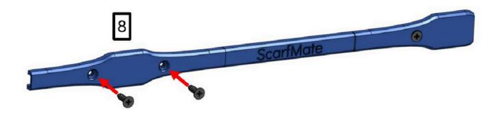
Step 8: Insert provided anchor in to hole's on middle connector & fasten it to the wall until anchor's bottoms out in the back of the middle connector
