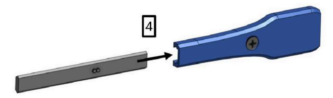
Step 4: With the (2) circles facing forward, insert back bar connector in to end piece until 1<sup>st</sup> circle snaps into place
