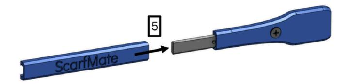
Step 5: With the <u>ScarfMate</u> logo facing forward, slide front bar connector over back bar connector until 2<sup>nd</sup> circle snaps into place
