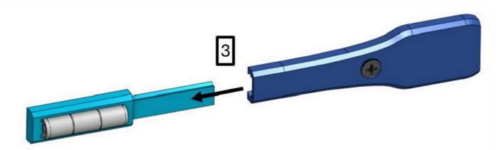
Step 3: Remove Level Holder from end piece to prepare for insertion of next section
