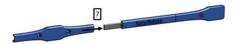
Step 7: With the back side facing up, slide a middle connector over the back bar connector until 2<sup>nd</sup> circle snaps into place
