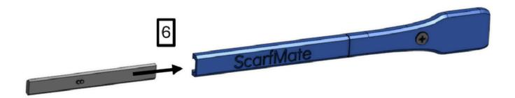
Step 6: With the (2) circles facing forward, insert another back bar connector in to front bar until 1st circle snaps into place
