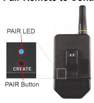
Press the remotes pair button on the back using a paperclip and the pair button on the front panel of the SCM-800. For additional information read the instruction manual provided with the remote. (Also can be found on our website: SimConSol.com)
