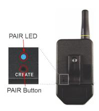
\*If the controller is only doing a single flash it is in slave mode and you must put it in administrator mode. To do this, hold down the pair button for 30 seconds at which time you will see a series of flashes from the blue pair LED. Now, when you press the pair button it should be doing a double flash indicating it is in administrator mode and ready to pair.
