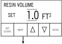
**Step 5I-B** –Set the amount of resin used in the system. The seven settings available are 0.4, 0.5, 0.6, 0.75, 1.0, 1.5, and 2.5 FT³. Use ▲ or ▼ to select value. Press NEXT to go to Step 6I-B. Press REGEN to return to previous step.
