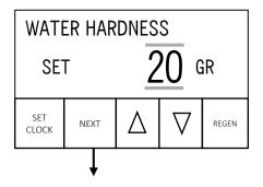
Step 6I-B — Set amount of water hardness present at water inlet. This setting is adjustable from 1 - 150 grains and is used in determining the volumetric capacity of the system. . Use ▲ or ▼ to select value. Press NEXT to go to Step 7I-B. Press REGEN to exit Installer Screen Settings.
