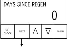
appear in 5 seconds the lock on the valve is activated. To unlock press ▼, NEXT, ▲, and SET CLOCK in sequence, then press ▲ and ▼ simultaneously for 3 seconds.
