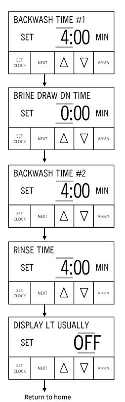
**Step 12I-A** – Select duration of 1st cycle. Use ▲ or ▼ to select value other than default value. Setting will flash when changed from this initial value. Press NEXT to go to Step 13I-A. Press REGEN to return to previous step.
