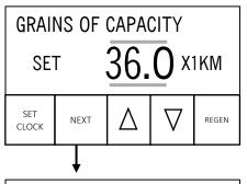
STEP 7I-A — Enter the ion exchange capacity in grains of hardness as calcium carbonate for the system based on test data using ▼ or ▲ buttons. Press NEXT to go to Step 8I-A. Press REGEN to return to previous step.
