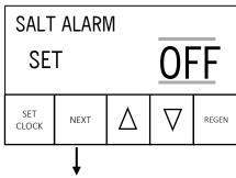
**Step 2M** – Set the Salt Alarm ON or OFF. Use ▲ or ▼ to select value. Press NEXT to go to Step 4M. Press REGEN to return to previous step.
