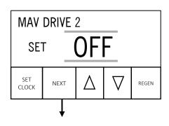
**Step 2I-R**— Select MAV DRIVE 2 output for use with NHWB or separate source backwash. Use ▲ or ▼ to select value other than default value
