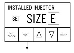
**Step 10I-B** – Select the size of injector to be used with the valve. Used in determining the duration of Brine Draw. Range is A – K. Use ▲ or ▼ to select value. Press NEXT to go to Step 11I-B. Press REGEN to return to previous step.
