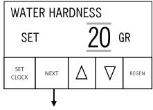
Step 8I-A – Set amount of water hardness present at water inlet. This setting is adjustable from 1 - 150 grains and is used in determining the volumetric capacity of the system. . Use ▲ or ▼ to select value. Press NEXT to go to Step 9I-A. Press REGEN to exit Installer Screen Settings.
