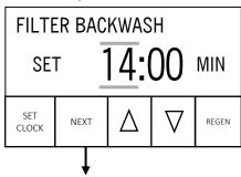
Step 5F – Select duration of Filter 1 2nd cycle. Only viewed if CHEMICAL-FREE FLT or FILTER is set in Step 2IF, when Filter 1 can be operated directly by the Valve Drive Motor. Use ▲ or ▼ to select value. Press NEXT to go to Step 6F. Press REGEN to return to previous step.
