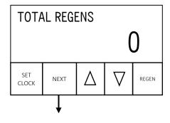
**STEP 5D** – Regenerations, total number since start-up: This display shows the total number of regenerations that have occurred since startup. Press NEXT to go to Step 6D. Press REGEN to return to previous step
