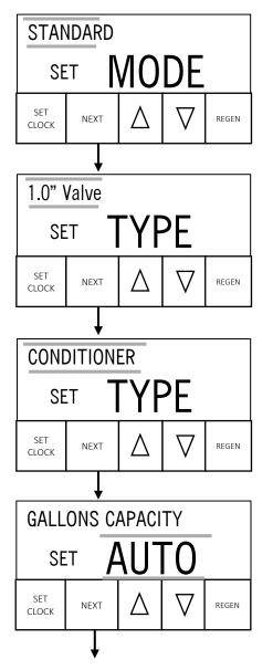
**Step 2I-A** – Set **STANDARD MODE**. Press NEXT to go to Step 3I-A. Press REGEN to exit Installer Screen Settings.
