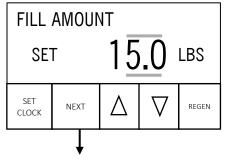
**STEP 11I-A** – Enter the pounds of salt per regeneration using ▼ or ▲ buttons. Press NEXT to go to Step 12I-A. Press REGEN to return to previous step
