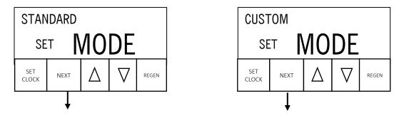
Step 2I-A – Set STANDARD MODE. Setting determines the normal operating parameters of the system. The three system types available are CONDITIONER, FILTER, and CHEM FILTER. Use ▲ or ▼ to select value. When STANDARD MODE is set follow the series of settings and steps for 3I-A. Press REGEN to exit Installer Screen Settings.
