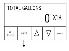
**STEP 4D** – Volume, total used since start-up: This display shows the total gallons treated since startup. This display will equal zero if a water meter is not installed. Press NEXT to go to Step5D. Press REGEN to return to previous step.
