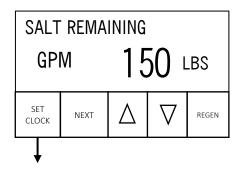
**Step 1-M2** – With the Salt Remaining display currently active, press SET to advance to Set Salt Level.
