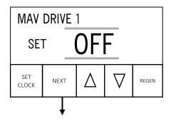
**Step 1I-R**− Select MAV DRIVE 1 output for use with NHWB or separate source backwash. Use **△** or **▼** to select value other than default value
