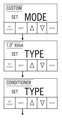
**Step 2I-B** – Set **CUSTOM MODE**. Press NEXT to go to Step 3I-B. Press REGEN to exit Installer Screen Settings.
