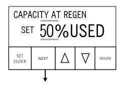
Step 9I-B – Set how much of the initial capacity may be used before the control would automatically trigger a regeneration cycle at the next regeneration time. Adjustable from 30 - 90% in 10% increments. Use ▲ or ▼ to select value. Press NEXT to go to Step 10I-B. Press REGEN to return to previous step.
