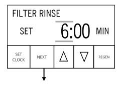
Step 6F – Select duration of Chemical-Free Filter 3rd cycle. Viewed only with CHEMICAL-FREE FLT set in Step 2I. In this cycle Aux MAV #1 is used to Air Charge the system. Use ▲ or ▼ to select value. Press NEXT to go to home screen. Press REGEN to return to previous step.
