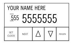
**STEP 1-M3** - Set phone number using the ▼ or ▲ arrow. Press NEXT to forward to the next digit. Press REGEN to return to previous digit.
