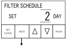
Step 4F – Select duration of Filter 1 1st cycle. Viewed only when CONDITIONERFILTER, CHEMICAL-FREE FLT, or FILTER is set in Step 2I. Use ▲ or ▼ to select value. Press NEXT to go to Step 5F. Press REGEN to return to previous step. DEFAULT = 21:00 MIN (CONDITIONER-FILTER), 14:00 (CHEMICAL-FREE FLT, or FILTER)
