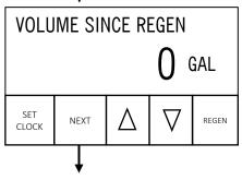
**STEP 3D** – Gallons, since last regeneration: This display shows the number of gallons that have been treated since the last regeneration. This display will equal zero if a water meter is not installed. Press the NEXT button to go to Step 4D. Press REGEN to return to previous step.
