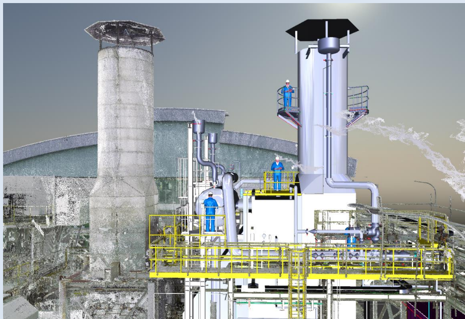
Final design model, with 3D laser scan
