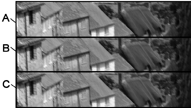
Fig. 9. Pictures of Goldhill showing 8 pixel standard motion blur in A, motion blur using a non-sequenced 32 element HC in B, and a sequenced encode in C.
