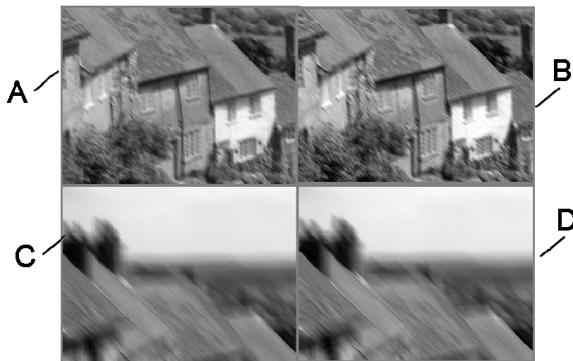
Fig. 11. Pictures A and C were encoded using a 512 element sequenced HC, and picture B and D represent typical staring array motion blur. Scene movement during image capture was 8 pixels for A and B and 32 pixels for C and D. There is no visible difference between typical motion blur and that obtained using sequenced Hadamard encoding.
