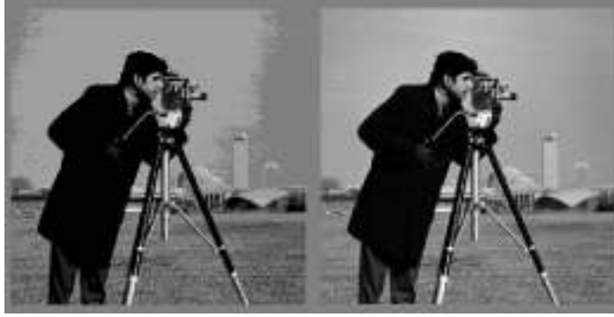
Fig. 4. Both the cameraman picture at left and the OCR reconstruction at right are digitized using 6 bits. The OCR picture has fewer quantization artifacts.
