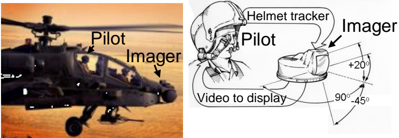
Figure 1.1. At left, the pilot is in the rear seat, and the imager is on the nose. As illustrated at right, the imager is in a turret that is directed in space by the pilot's head. The video from the nose is fed back to a display on the pilot's helmet. He sees the image only in his right eye.
