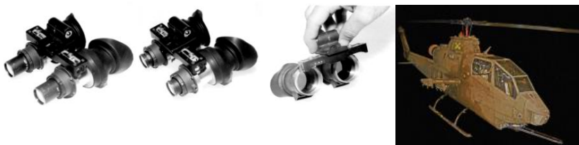
Figure 1.8 shows direct view goggles fabricated to test various combinations of FOV and image resolution. The aviator subjects flew from the front seat of a Cobra.
