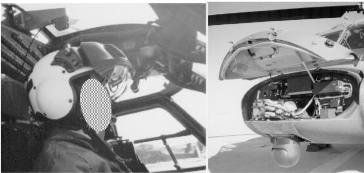
Figure 9.3 showing the thermal system used to demonstrate the effect of field replication on pilotage imagery.
