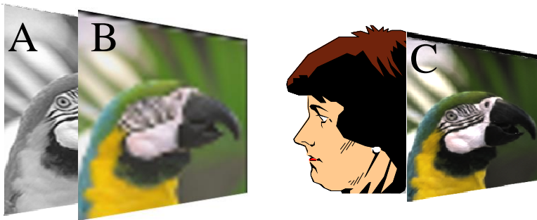
Figure 3. A high resolution monochromatic picture (A) is viewed through a semi-transparent, blurred color picture (B). The person sees a high resolution color image (C). Multiplying A and B pixel by pixel gives the same result.
