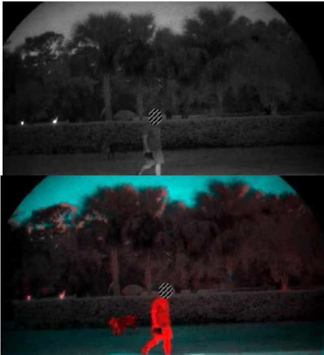
Figure 6 shows color processing using a low resolution (128 by 94 pixel) thermal image as the color red.
