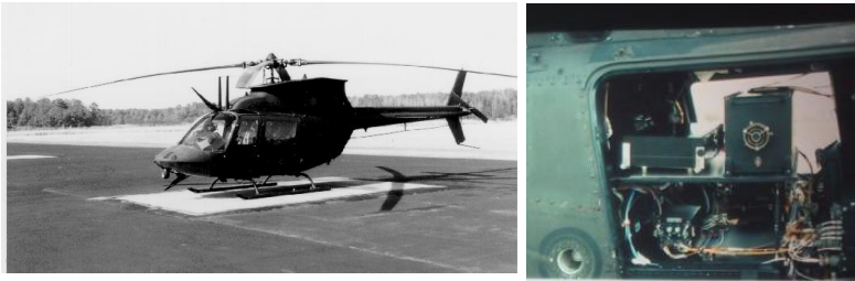
Figure 10.1 The Test Aircraft is an OH-58D with the Mast Mounted Sight removed. The accelerometer monitoring and data recording equipment was mounted in back as shown.
