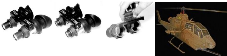
Figure 7.1 shows direct view goggles fabricated to test various combinations of FOV and image resolution. The aviator subjects flew from the front seat of a Cobra.
