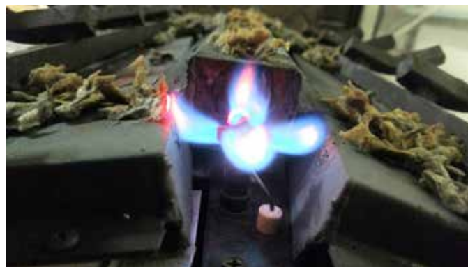
Figure 4.3 IPI Pilot Flame Patterns
