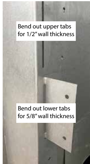
Figure 6.4 Nailing tab bent out for installation
