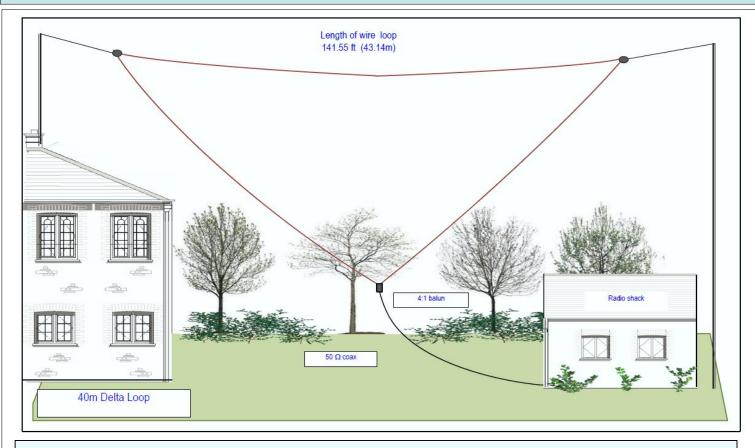
This simple broad band antenna is easy to build, has gain similar to that of a dipole and is tolerant of nearby objects. It can be erected in almost any configuration provided the wires are well separated otherwise it acts as a singe band broadband dipole. I generally feed it in the centre at the bottom but a side can be used to give vertical polarisation, as in a 4 sided quad. The gain over a dipole is claimed to be about 2db.
