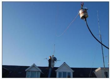
Pictures of the inverted Delta Loop as installed in the Garden in sunny Guernsey. Note that the coax from the bottom of the balun is tied to the wooden garden structure to prevent the antenna swaying into the bushes during high winds.
