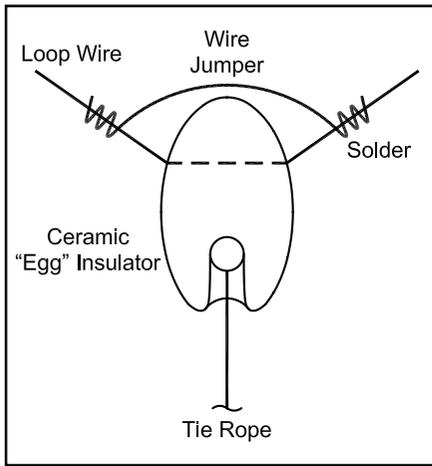
Figure 4—One simple method of attaching tie ropes to wire antennas.
