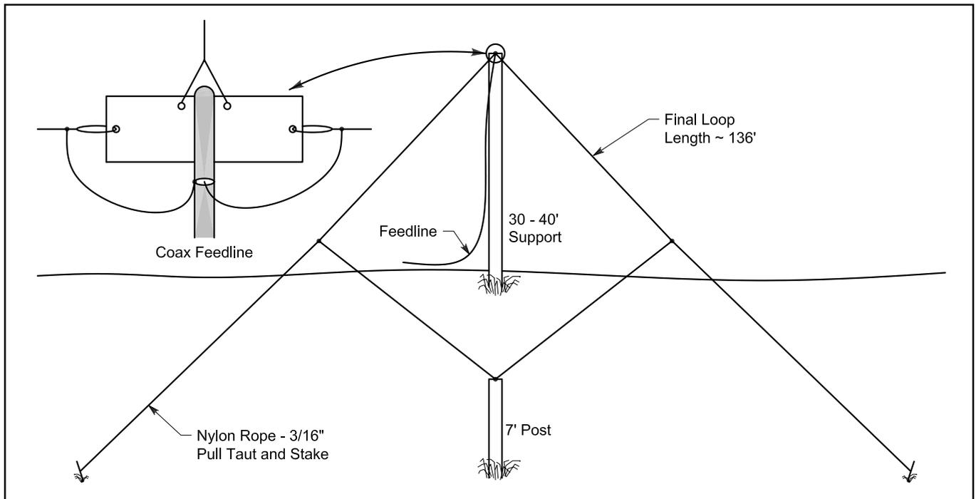
Figure 3—The vertical support of the Single-Masted Sloop can be a mast, tree, building, flagpole, and so on. The simplicity of the design and the multidirectional gain delivered at the harmonics make this antenna a good candidate for Field Day.
