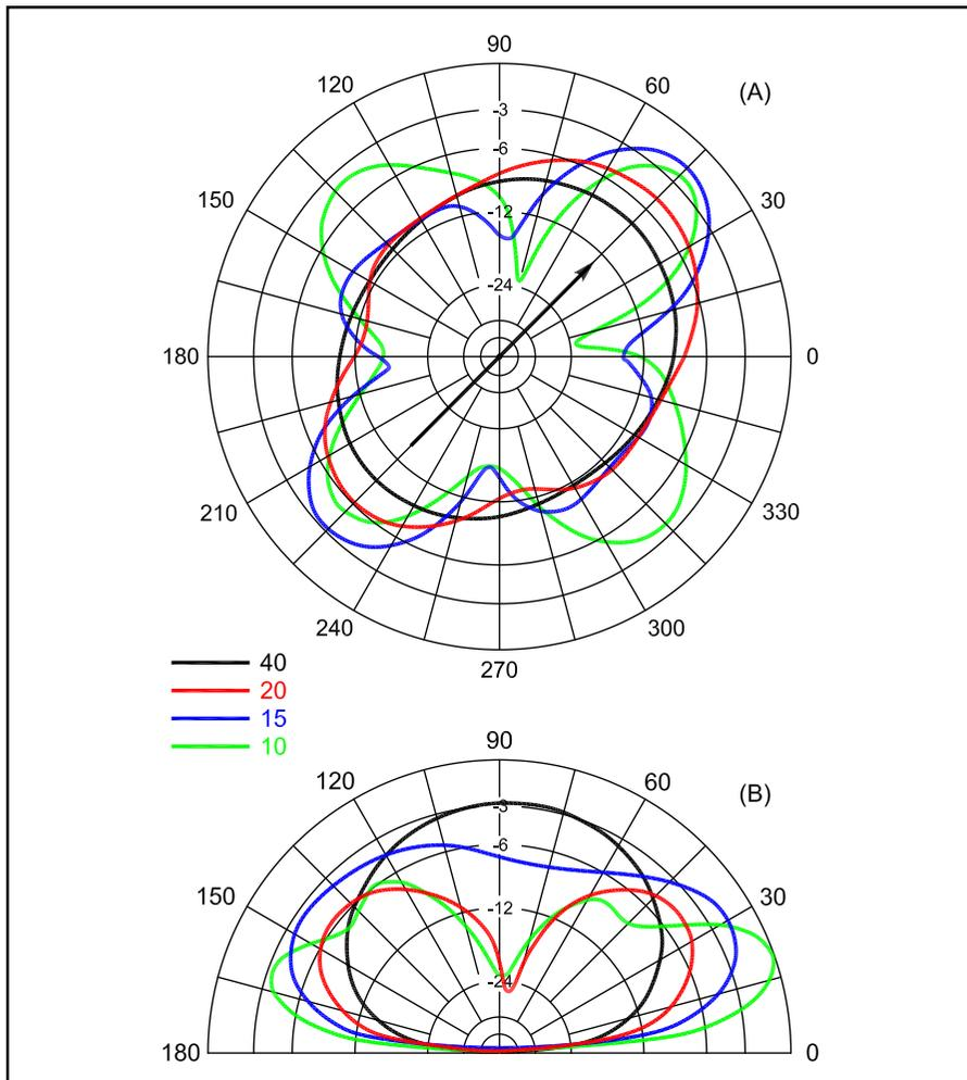
Figure 2—EZNEC study of the far field radiation patterns of the 40 through 10-meter “Sloop.” The arrow indicates the direction of the slope. A is the azimuth plot at 30 degrees elevation. B shows the elevation plot along the axis of maximum gain, 45-225 degrees.
