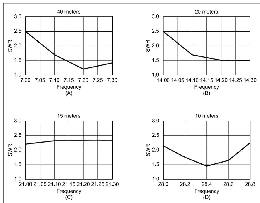
Figure 1—SWR vs. frequency plots for the 136-foot, 40 through 10-meter sloop. The SWR minimum for the four bands is easily adjusted by adding or deleting small lengths of wire from the loop.
