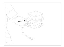
Pull out the shaft. Clean it with small brush from the salt remains. Look into the hole, where was shaft and remove salt from there too.
