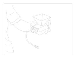
Pull up fixator of shaft. Now you can pull out the main part of salt feeder. Be careful, there are left some salt inside and do not let it fall on the floor.
