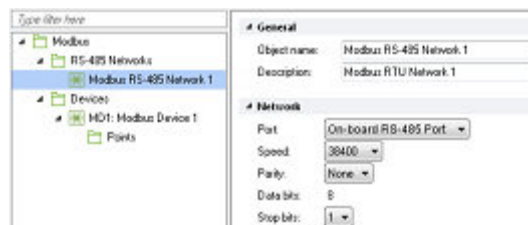
Figure 149: Setting the Modbus Network Communication Parameters in EC-gfxProgram's Resources Configuration Window
