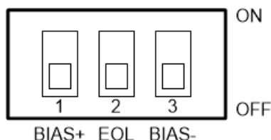
Figure 151: Typical ECLYPSE Controller with Separate EOL Termination and Bias Configuration Settings
