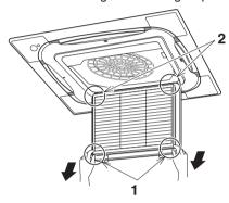
1 Pull the air filter end inclined downward and unhook the hooking hole of the air filter from the projection of the grille. (Both right and left)
