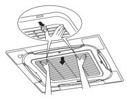
Remove the straps of the suction grille.Remove the two straps holding the main part of the panel.
