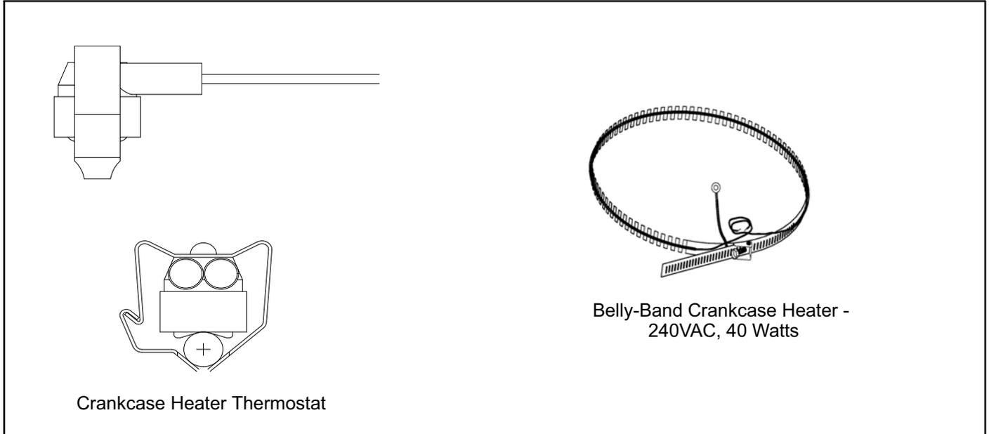
**Figure 35. Belly-Band Crankcase Heater Thermostat**
