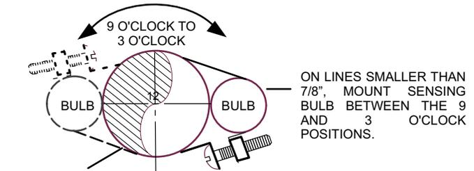
ON LINES SMALLER THAN 7/8", MOUNT SENSING BULB BETWEEN THE 9 AND 3 O'CLOCK POSITIONS.
