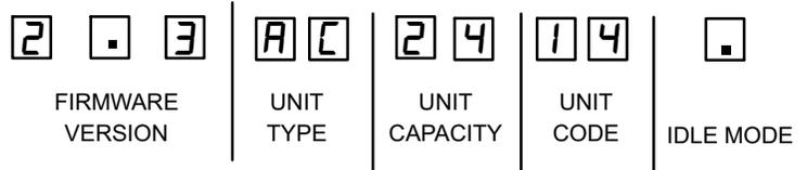
**Figure 15. Outdoor Control 7-Segment Unit Status Displays**
