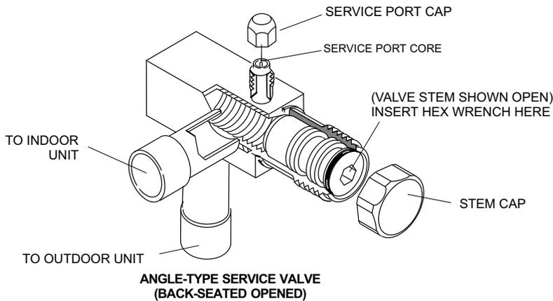
When service valve is **OPEN**, the service port is open to line set, indoor and outdoor unit.
