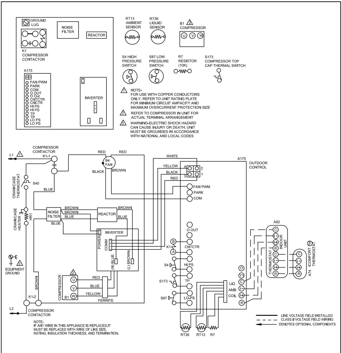
Figure 23. Typical Unit Wiring (XC20-048 and -060)
