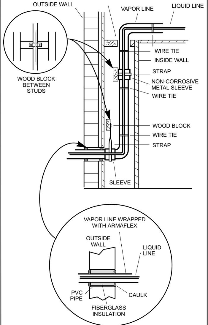
*NOTE* - SIMILAR INSTALLATION PRACTICES SHOULD BE USED IF LINE SET IS TO BE INSTALLED ON EXTERIOR OF OUTSIDE WALL.
