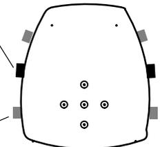
ONE BRACKET PER SIDE (MIN.); FOR EXTRA STABILITY, TWO BRACKETS PER SIDE, 2" (50.8MM) FROM EACH CORNER.
