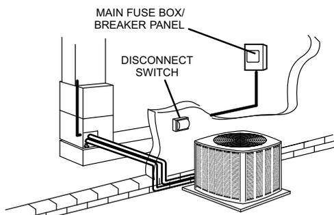
**NOTE** - UNITS ARE APPROVED FOR USE ONLY WITH COPPER CONDUCTORS. GROUND UNIT AT DISCONNECT SWITCH OR TO AN EARTH GROUND.
