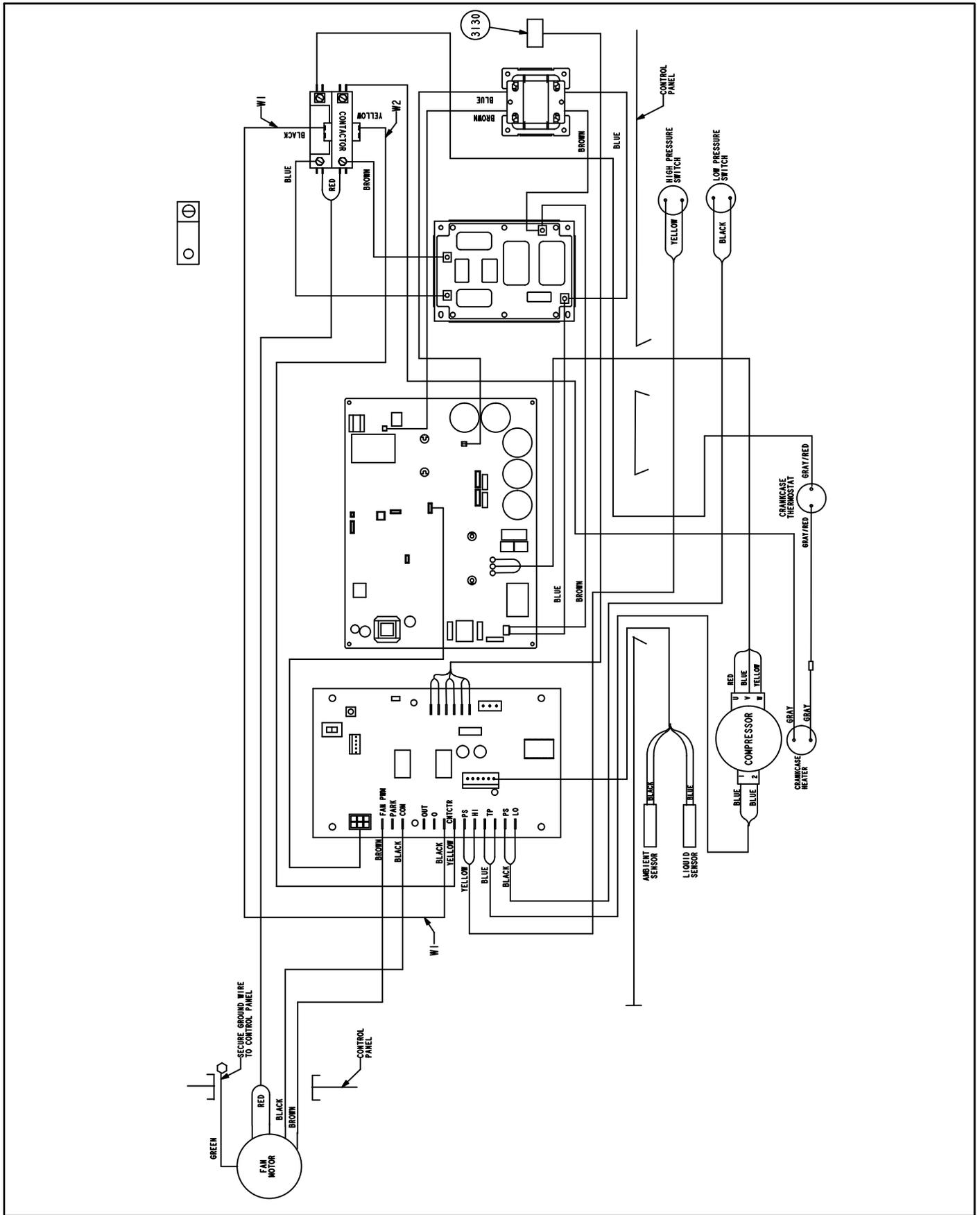
Figure 26. Typical Factory Wiring (XC20-048 and -060)
