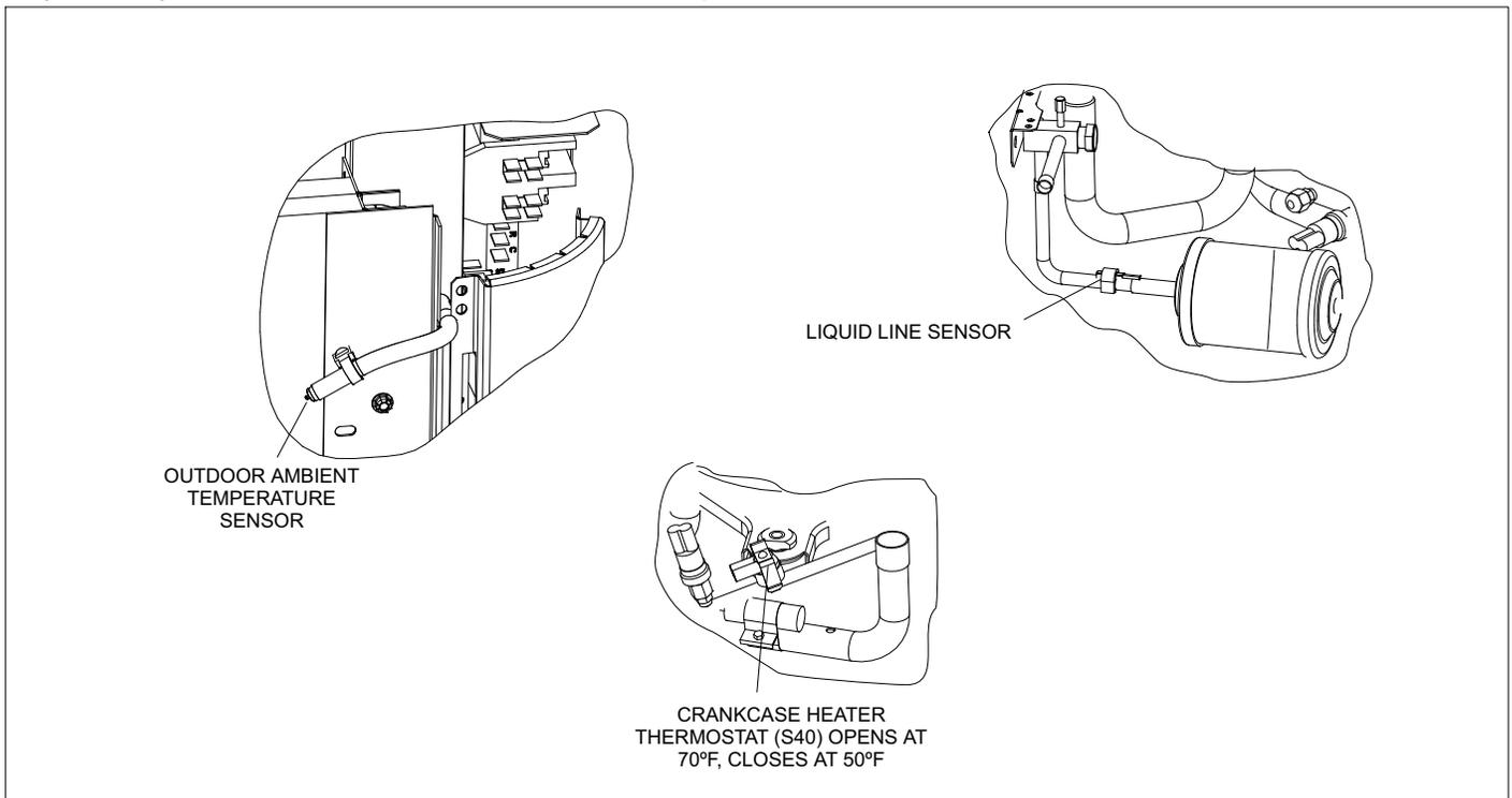
**Figure 50. Temperature Sensor Locations**
