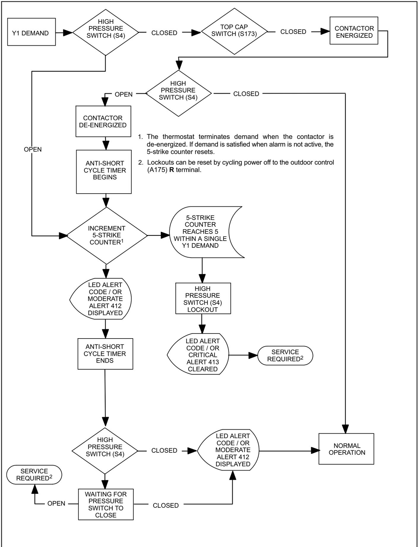
Figure 29. High Pressure Switch (S4) Sequence of Operation (All Versions)
