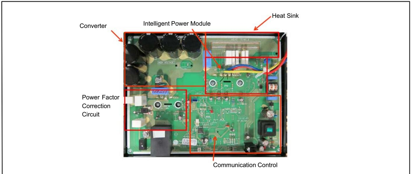
**Figure 52. 4- and 5-Ton Unit Inverter**
