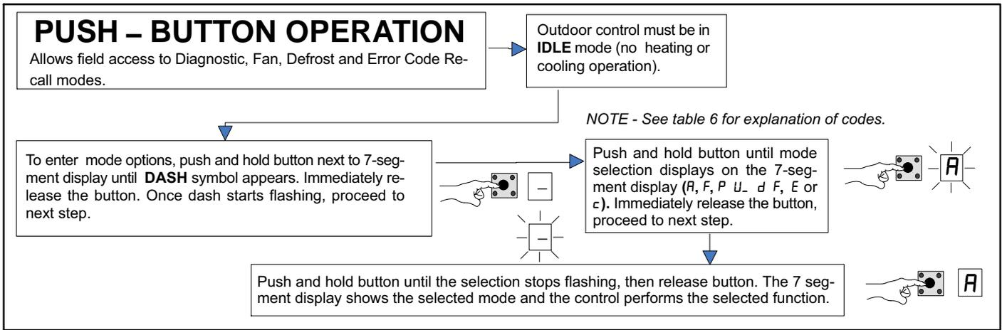
**Figure 16. Push-Button Operation**
