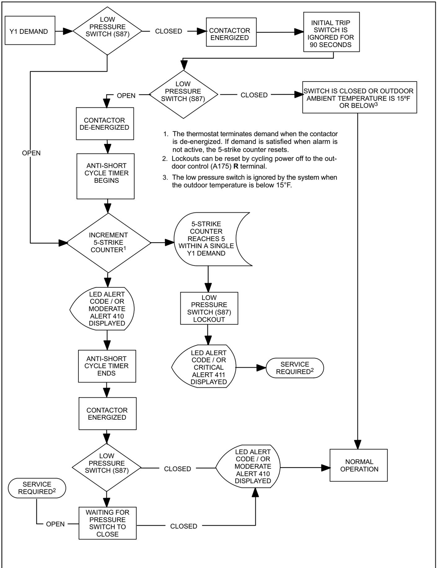
Figure 28. Low Pressure Switch (S87) Sequence of Operation (All Versions)
