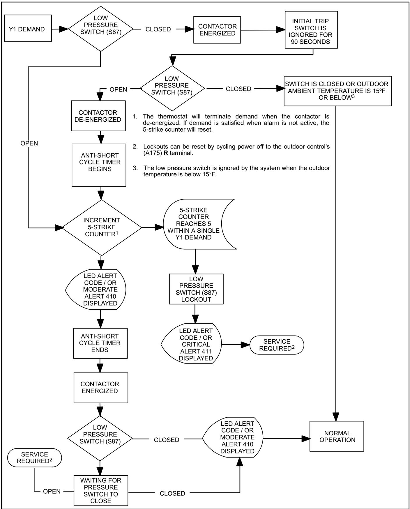
Figure 31. Low Pressure Switch (S87) Sequence of Operation (All Versions)
