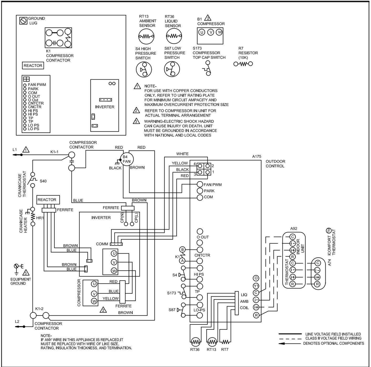
Figure 22. Typical Unit Wiring (XC20-024 and -036)
