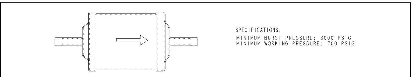
**Figure 39. Liquid Line Filter Drier**
