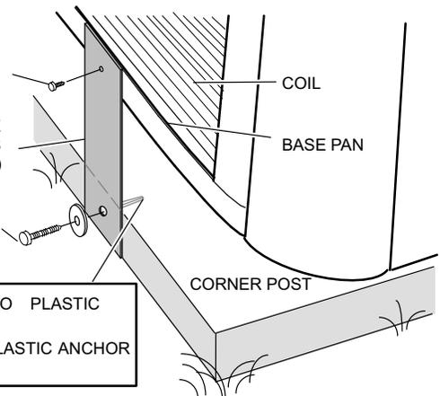
**CONCRETE SLAB** — USE TWO PLASTIC ANCHORS (HOLE DRILL 1/4")
