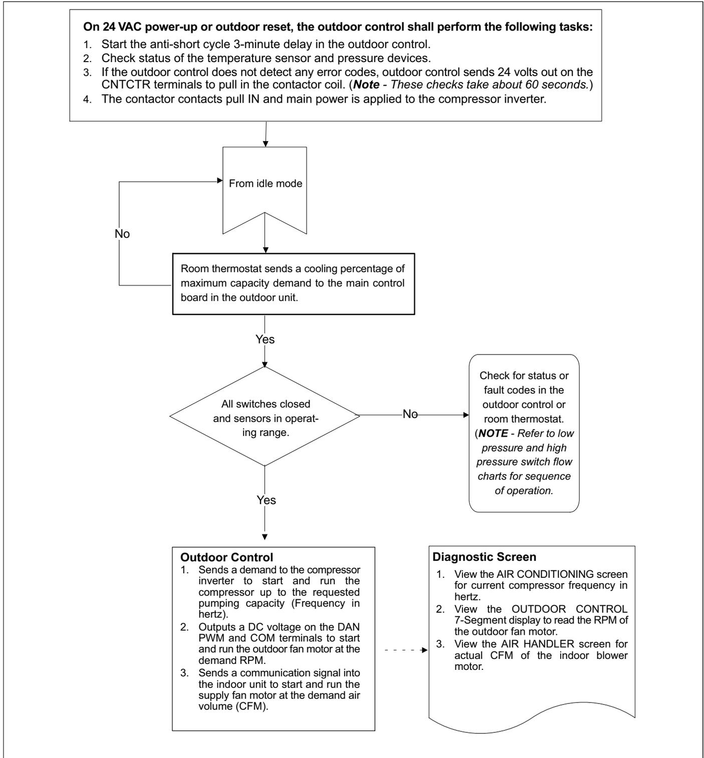
Figure 27. 24 Volt Power-Up or Outdoor Reset
