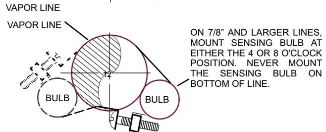
ON 7/8" AND LARGER LINES, MOUNT SENSING BULB AT EITHER THE 4 OR 8 O'CLOCK POSITION. NEVER MOUNT THE SENSING BULB ON BOTTOM OF LINE.
