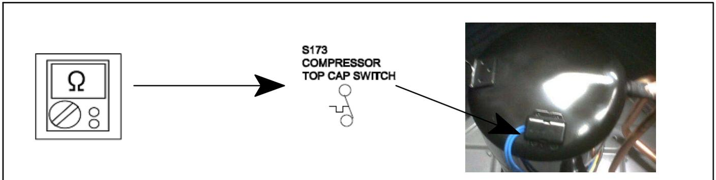
Figure 41. Verifying Top Cap Thermal Sensor Switch
