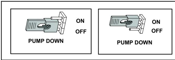
**Figure 17. Pump-Down Jumper**
