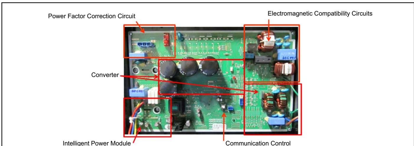
**Figure 51. 2- and 3-Ton Unit Inverter**
