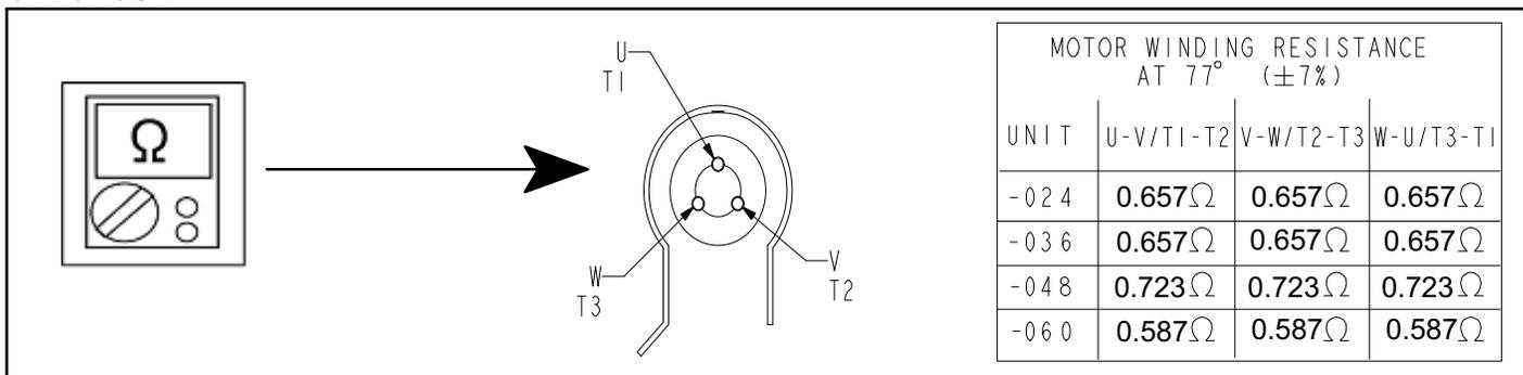
**Figure 33. Compressor Operation, Checkout and Status/Error Codes**
