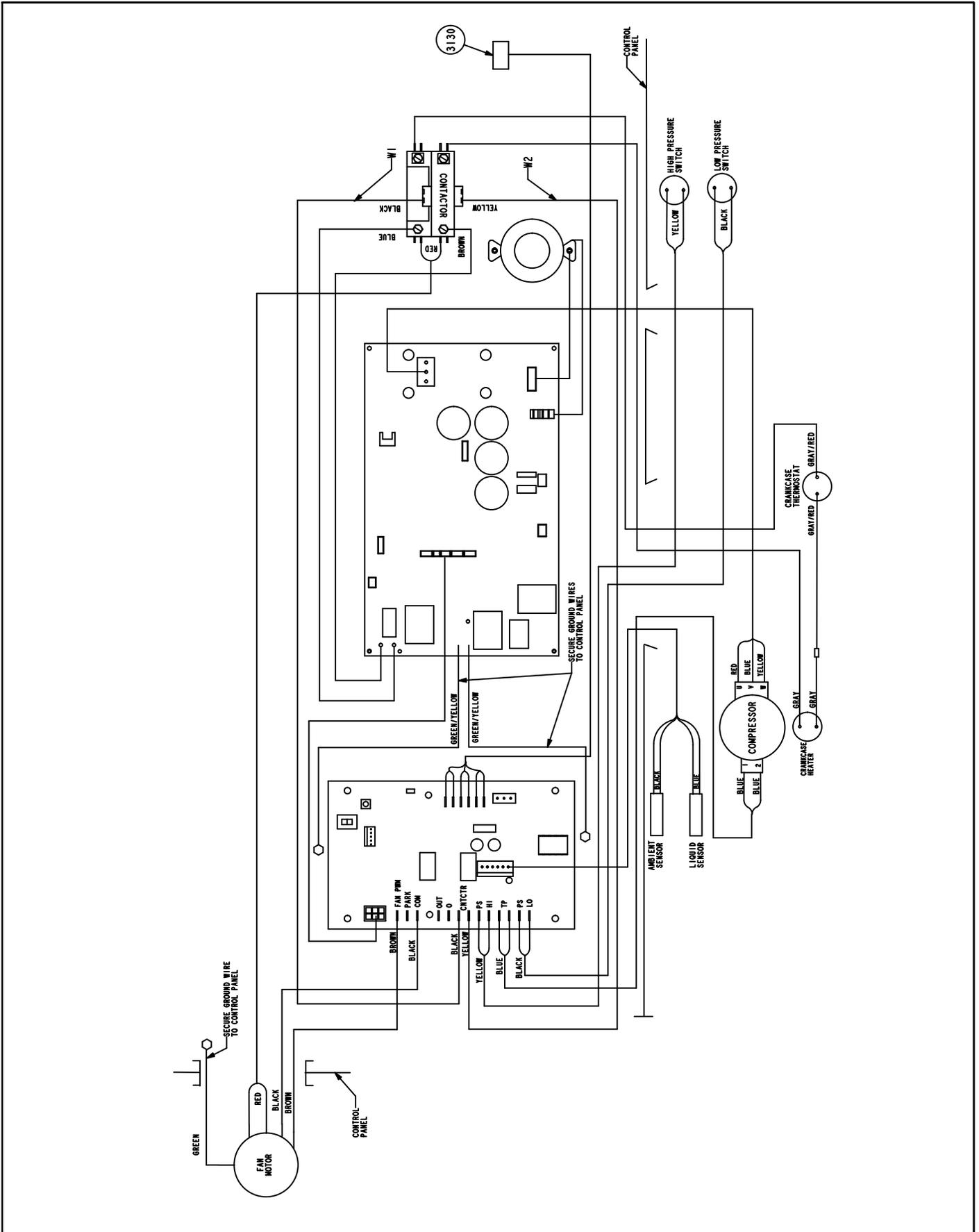
Figure 25. Typical Factory Wiring (XC20-024 and -036)
