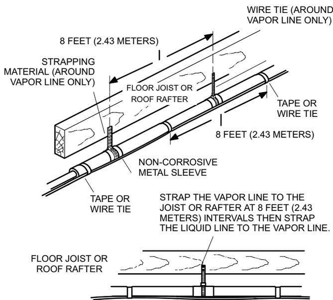
**IMPORTANT** - Refrigerant lines must not contact structure.
