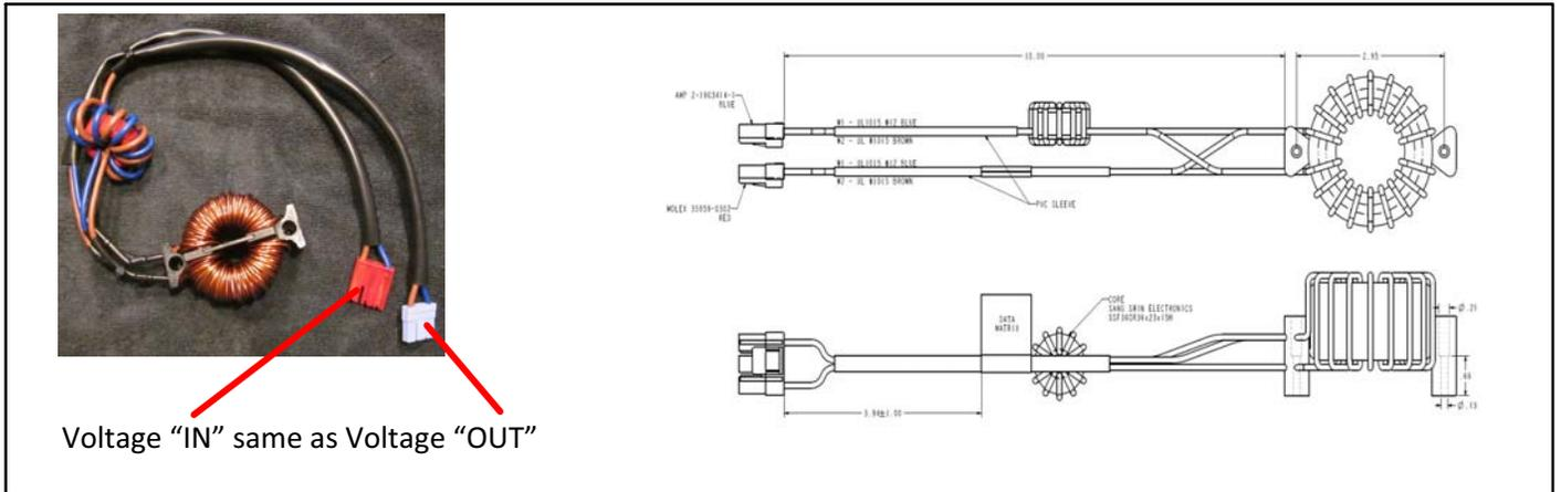
**Figure 42. XC/XP 20-024 and -036 Reactor**
