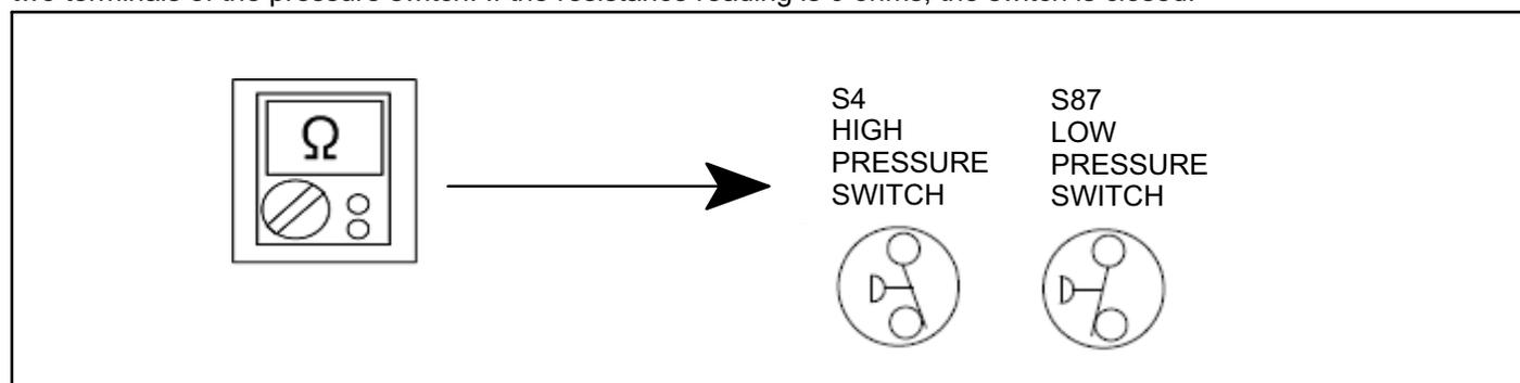
**Figure 30. Verifying High Pressure and Low Pressure Switch Operation**
