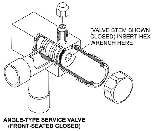
When service valve is **CLOSED**, the service port is open to the line set and indoor unit.
