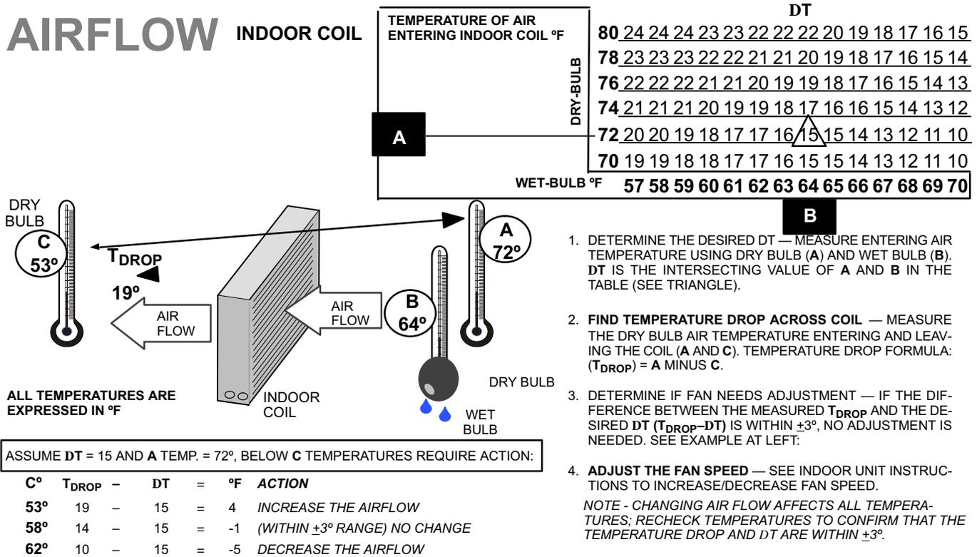
Figure 55. Checking Indoor Airflow over Evaporator Coil using Delta-T Chart
