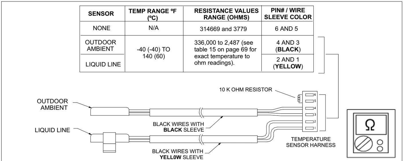
**Figure 49. Temperature Sensor Specifications**
