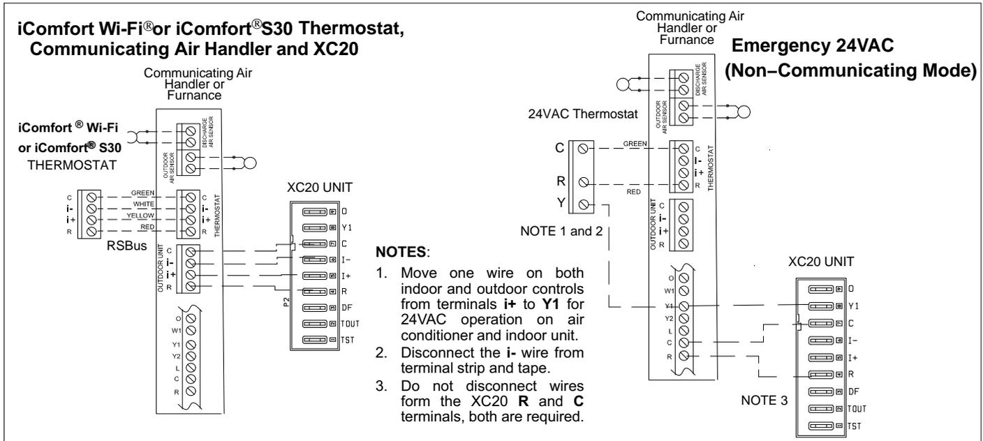
Figure 53. Emergency 24VAC System Operation
