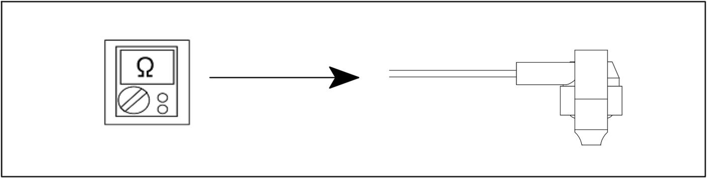
**Figure 37. Checking Crankcase Heater Thermostat**
