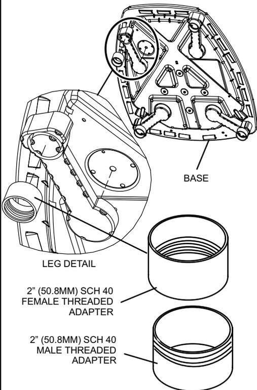
USE ADDITIONAL 2" SCH 40 MALE THREADED ADAPTERS WHICH CAN BE THREADED INTO THE FEMALE THREADED ADAPTERS TO MAKE ADDITIONAL ADJUSTMENTS TO THE LEVEL OF THE UNIT.
