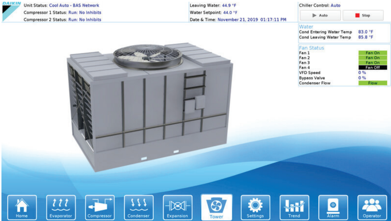
Figure 50: Cooling Tower Information
