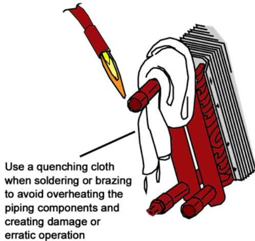
Figure 6: Protect Components from Overheating
